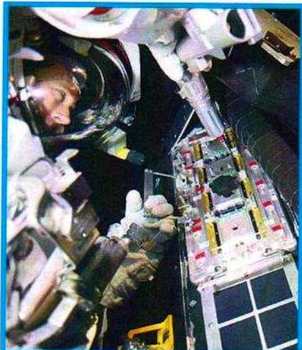
Astronaut Andrew Feustel practices installing the Fastener Capture Plate on an underwater mock up of the Advanced Camera for Surveys at the Neutral Buoyancy Laboratory in Houston. Astronauts will attempt to repair the instrument during Servicing Mission 4 to Hubble.
