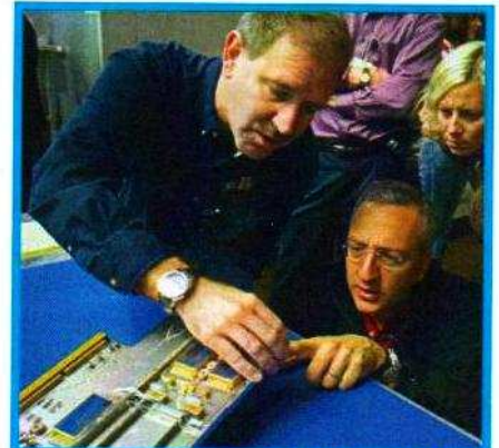
Astronauts John Grunsfeld (L) and Mike Massimino and a team of Hubble engineers inspect position indicator decals on the STIS replacement printed circuit board. The board will be installed during Servicing Mission 4 in an attempt to restore power to the instrument.
